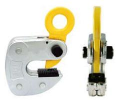
This HLC clamp is used for horizontal lifting and transfer of steel plates and is particularly suited to this application due to the special thin ground plate and buffer cams which facilitate easy insertion and removal under the plate being lifted. It can also be used hanging vertically under a spreader.
